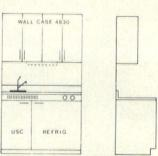
Models show thoughtful details Dwyer didn't have to change: seamless porcelin-on-steel counters; concealed hinges; and appliance doors that match cabinets. Inside shelves roll out. All components can be rearranged for the customer.
