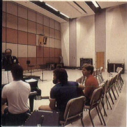
Large practice rooms for choir, orchestra and band (left), are designed to approximate acoustical conditions found during an actual performance. Fabric mounted panels on the walls take the place of the audience.
