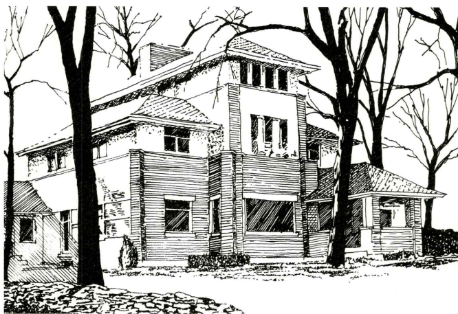
The Rollin Furbeck house by Frank Lloyd Wright (left) features a central vertical mass, an entry-way sheltered by its own roof structure, and a change in material below the second floor windows. The Barbour residence (right) interprets these elements, but replaces the horizontal window banding with a grid.
