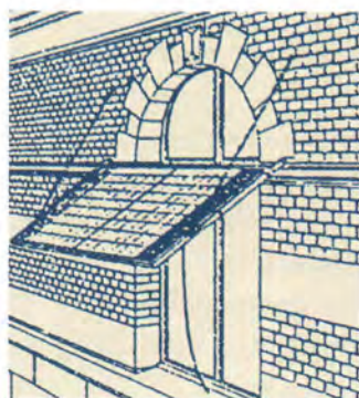
Prismatic transoms on the Hamm Building (top), and illustration of Luxfer Prism from 1902.
