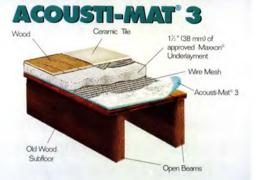
Increases IIC and STC up to 17 rating points over wood frame and increases IIC more than 20 rating points over concrete
