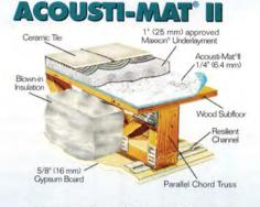
Increases IIC and STC up to 10 rating points over wood frame and increases IIC up to 20 rating points over concrete
