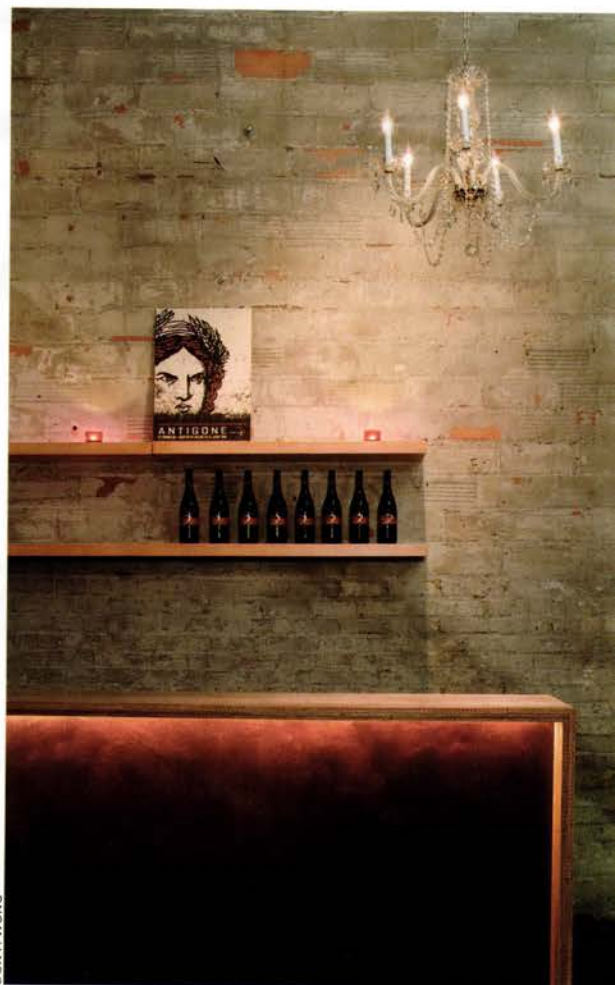
Previous spread and above: Jeune Lune's set builders constructed the simple, elegant furniture—tabletops, shelves, benches, and the 30-foot-long bar—from birch-veneer plywood and MDF. Opposite: The new graphics board displays the company's Tony Award in a simple case, along with museum-style letter transfers highlighting the upcoming season.
