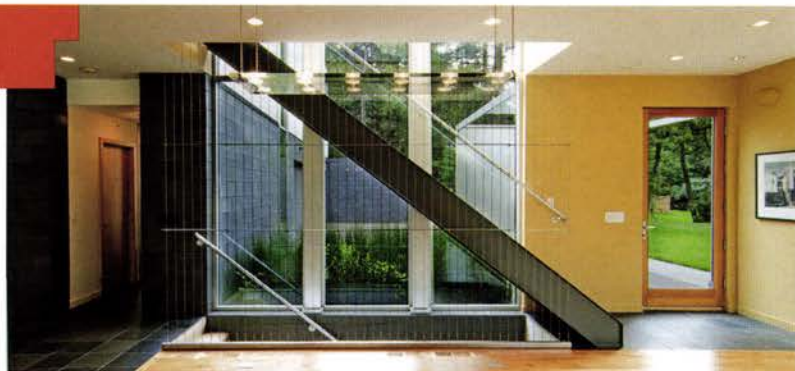
Taut stainless-steel cables take the place of conventional stair railings at the home's front entry. A two-story window looks out onto the entry court and draws natural light into the dining area.
