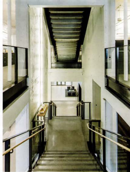
In HGA's hands, the Ford Center's original Model T showroom became a dramatic reception and gallery space with a row of flexible meeting rooms. The central staircase sits in the old elevator shaft that used to carry cars down the plant's vertical assembly line.
