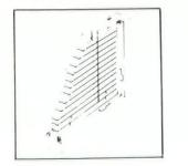
**SLIMSHADE**<sup>®</sup> – Only Pella Windows offer this economical and practical means of light and sun control, Slimshade is a narrow-slat blind set inside the sash between exterior glazing and the double glazing panel, as shown in the drawing.
