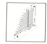
SLIMSHADE® – Only Pella Windows offer this economical and practical means of light and sun control. Slimshade is a narrow-slat blind set inside the sash between exterior glazing and the double glazing panel, as shown in the drawing.
