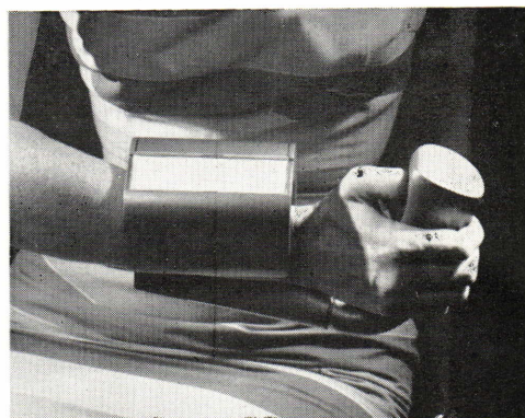
This mechanism worn on the wrist is activated by digital and wrist motions. The printing mechanism fits inside "wrap-around" and prints sheets from behind.
