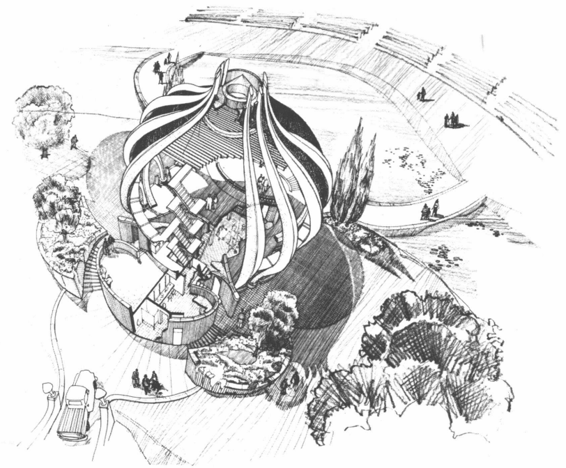
A bird's eye, cut-away section shows the roof dome, gridiron level and fly loft, and the catwalk above the stage level, service room and deck. Below are the scenery shop and the dressing rooms.
