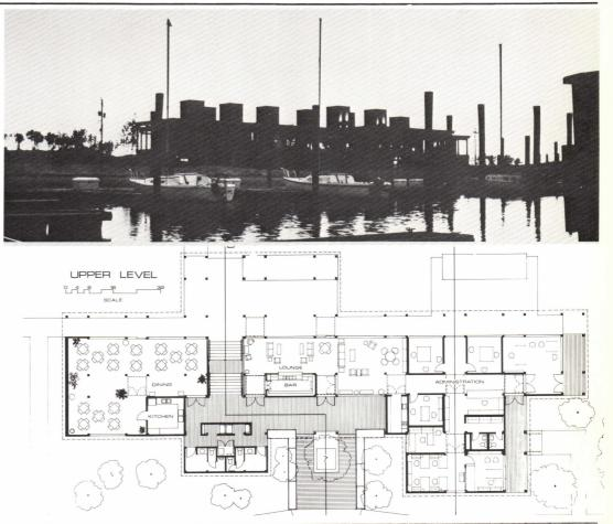
way, the pilings are placed on a grid of varying sizes—eight, 12 and 16 foot bays—to allow support for both large and small spaces as the building changed. The entire system is what the architect calls an "enclosed pier."
