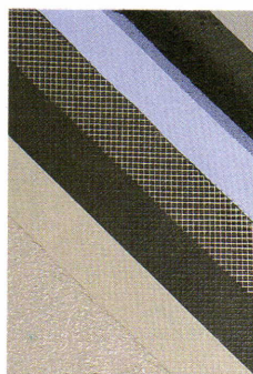
A. STO Flexyl Adhesive/Waterproof B. STYROFOAM® Brand Insulation C. STO Flexyl with STO Primer D. STO Reinforced Fiberglass Mesh E. STO Finish
