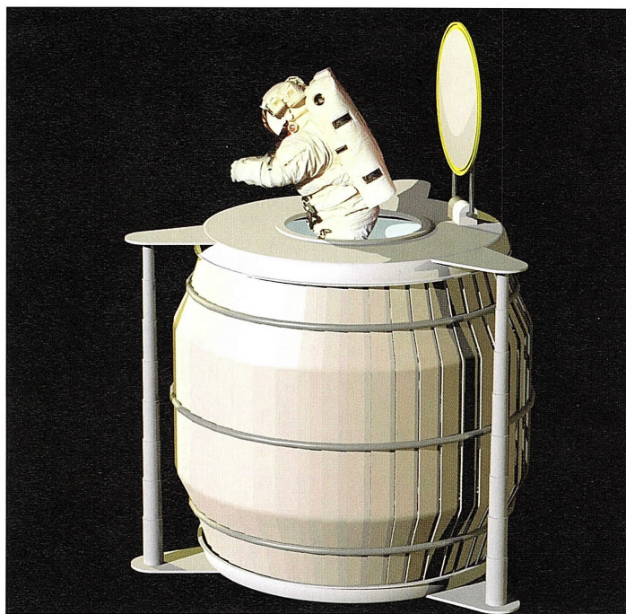
The Advanced Inflatable Airlock, to be used by astronauts performing spacewalks, was designed for NASA by FTL in collaboration with Honeywell
