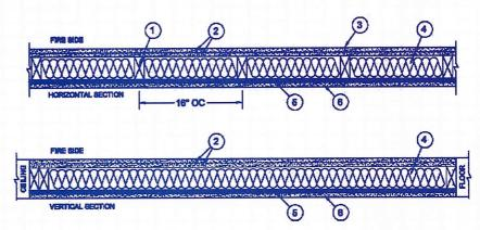
Pyro-Guard pressure impregnated fire-retardant-treated wood can be used in lieu of steel and concrete in noncombustible types of construction. Pyro-Guard does not require water or electricity to protect the wood and therefore provides passive protection. When properly installed according to code requirements, Pyro-Guard fire-retardant-treated wood never needs additional inspection or service and is free of these ongoing maintenance costs.
