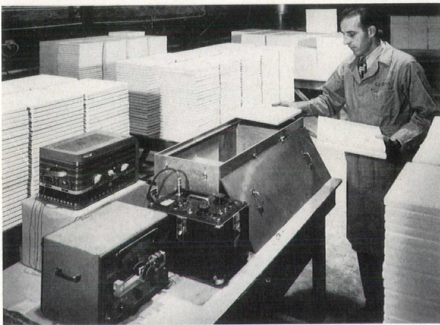
Sound equipment used to test acoustic properties of paint tile.
