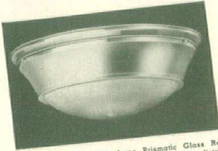
No. 3355—Surface type, Holophane Prismatic Glass Refractor provides a widespread symmetrical pattern light distribution. Spacing up to 2.0 times the mounting height above surface to be lighted provides uniform illumination.
