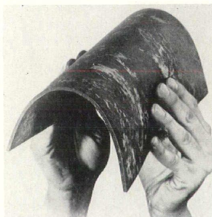
(Above) "Terraflex," the new J-M Flooring material is extremely flexible. When slightly heated, it can be curved to form stair nosings and coved bases. This characteristic also permits the floor to conform to any uneven surfaces and provided unusual resilience and comfort under foot.
