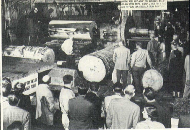
Peeling of veneer at Simpson Logging Company's Olympic plant in Shelton was part of the full-day demonstration of wood products practices presented for the A.I.A. convention delegates who toured Mason County.
