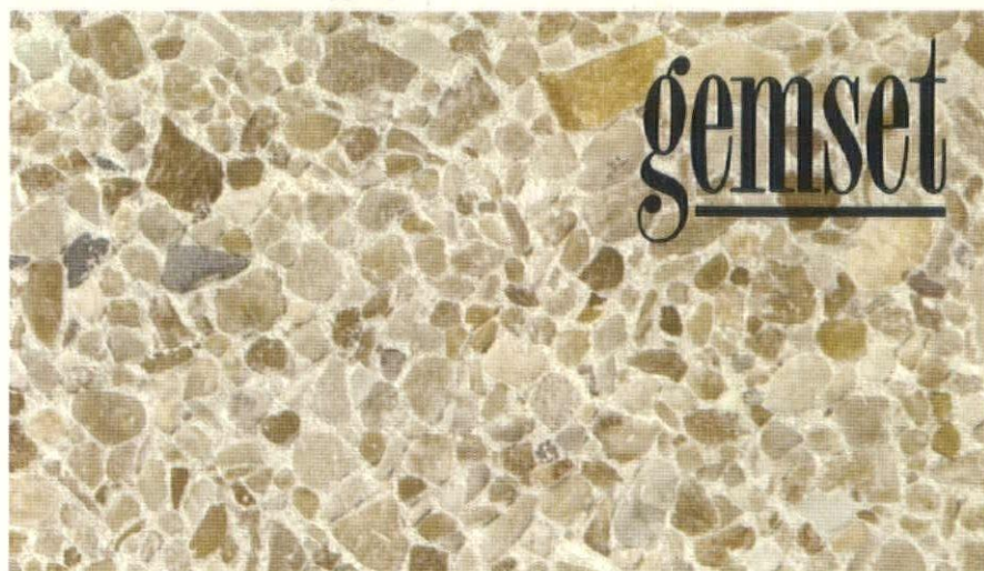
No. B136—river gravel aggregate (retarded matrix)
