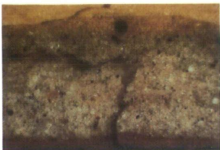
• Paint cross section, photographed at 220X, taken from helmet of miner, Science Revealing the Treasures of the Earth . Note horizontal and vertical cracks.
