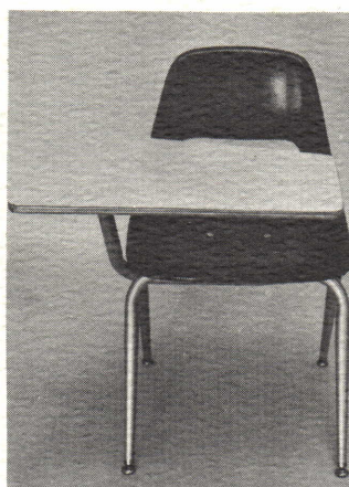
CHAIR/DESK. Student's-13 ga. and 16 ga. tubular steel frame w/oven baked enamel finish; nylon floor glides. Fiberglass bucket seat, wall saver design. Hot pressed plastic laminated, trapezoidal 17" x 12" x 22", tablet arm with backing sheet.
