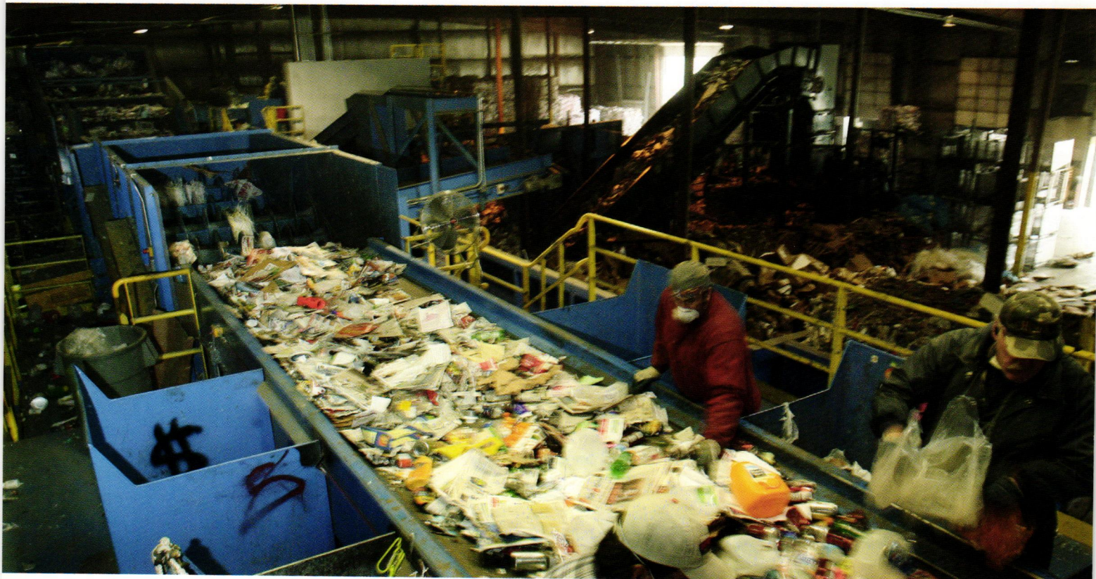
Contaminates are sorted from the Single Stream machine at Millennium Recycling
