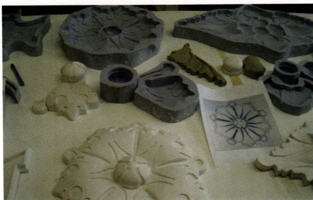
Plaster medallions were cast in rubber molds.
