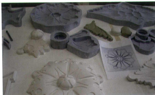
Plaster medallions were cast in rubber molds.
