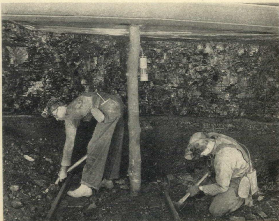
Below: Miners at the "face" working on track. Note protective hats and shoes, approved electric cap lamps, and self-rescuers.
