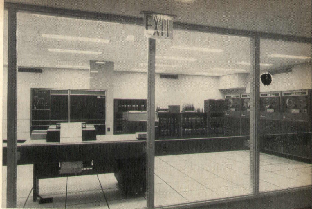
View of computer center through the surrounding interior glass wall which protects the delicate machinery and maintains the appropriate operating temperature.
