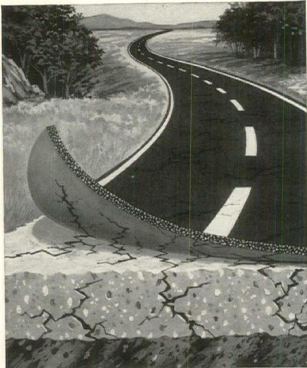
**CEMENT BASE BREAK-UP** is usually the real problem at the bottom of crack reflection. Cement-treated bases develop shrinkage cracks which eventually reflect through the protective riding surface. As these cracks increase in number and size, surface water enters, thereby causing more distress from instability and freeze-thaw action. Stronger, economical all-Asphalt pavement construction in the first place is the common-sense answer to all road- and street-building problems.
