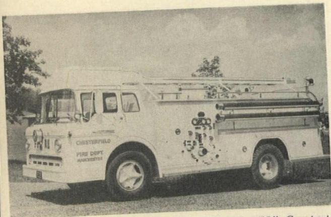
Ford Model C-750 with Tilt Cab Forward, "FL" Compartments, Overhead Ladder Carrier, Model CM-750 Waterous Two-Stage Pump & Waterous CP-1 Power Take-Off Pump. (Oren Roanoke Corp.)
