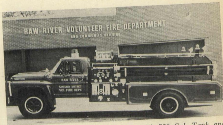
At left, C850 Ford, 750 GPM Pumper with 750 Gal. Tank and twin electric booster reels, now in service, and above, John Bean 500 GPM, pumper tanker with 860 gal. tank. (Jack L. Slagle Fire Equipment Co., Inc.)
