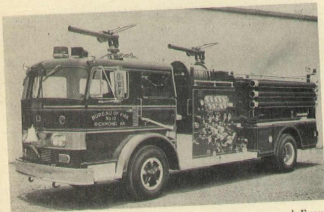
Oren Guardian Model 1002 Combination Pumper and Foam unit. Waterous 1000 GPM Two Stage Centrifugal Pump. When all outlets are Employed Unit Capable of Producing a minimum of 12,000 GPM Expansion Foam (Oren Roanoke Corp.)
