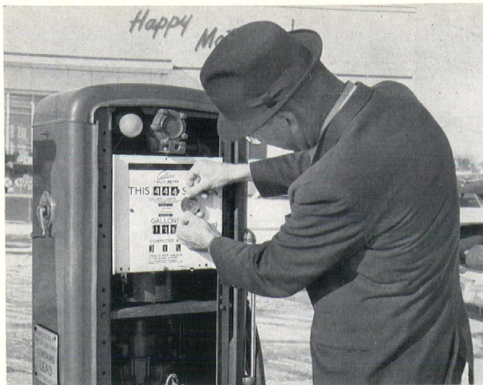
A weights & measures inspector places the department seal on this gasoline tank to denote that it has been tested and approved for accuracy in metering that product.
