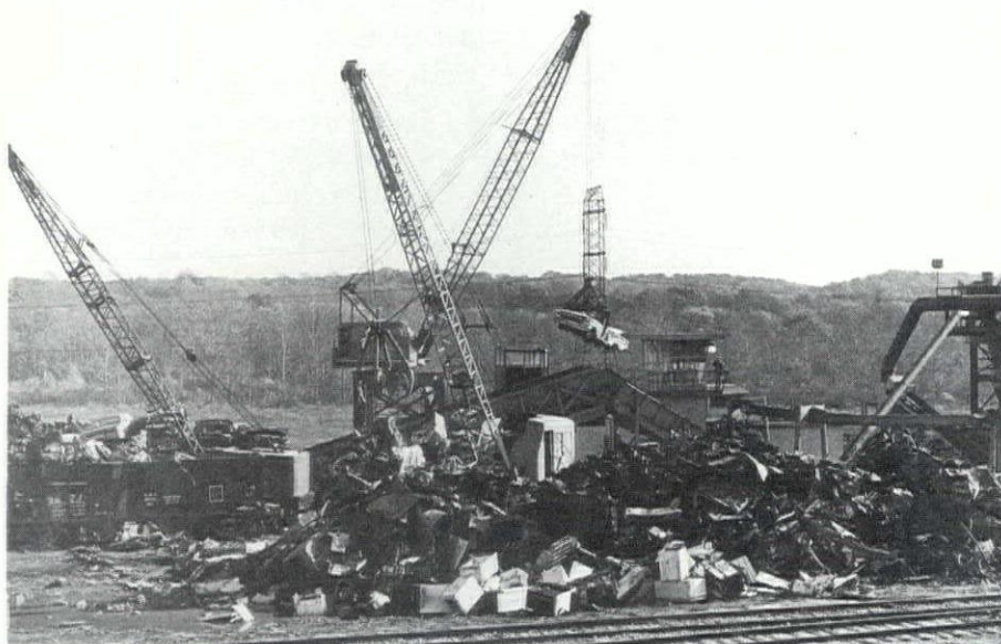
From worn out washing machines to smashed up old cars . . . Peck processes for re-use more than 240 million pounds of metal materials each year for mills and foundries throughout the U.S. The car above is being placed in the fragmentizer. In less than 60 seconds it will become 1,500 pounds of steel ready for use again at the mill.
