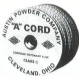
Austin Detonating Cord travels at the rate of better than 20,000 feet per second along its entire length . . . is offered in grades that possess more than enough strength to initiate an entire column of explosives, blasting agent primers and even some blasting agents.
