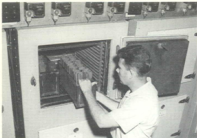
Seed inspection is one of the many services of the Department. To test the rate of germination, seeds are treated and wrapped in dampened paper and then placed in germination chambers which offer the seed optimum growing conditions.
