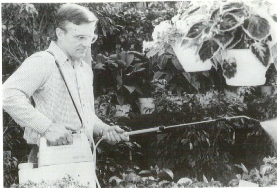
The country's first battery-operated garden sprayer, the Toyoset ESD-5, offers an alternative to the old bottle and hose method.
