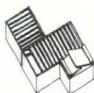
2. Sections are cut apart and placed with crane.
