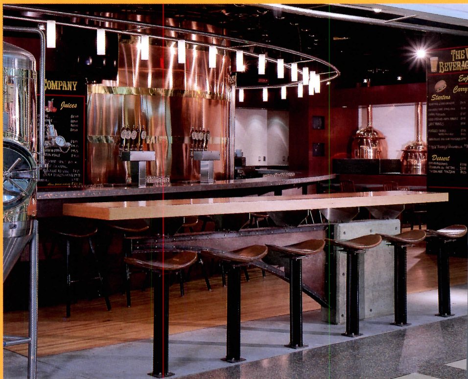
For a pub at Washington National Airport, Jameson conferred with the cement manufacturer to develop the proper mix for a countertop to include copper and tempered glass.
