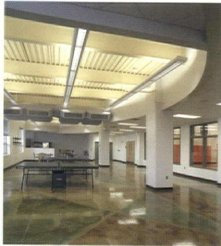
Ample daylighting reduces dependence on artificial lights (above). Much of the flooring is stained concrete (left).
