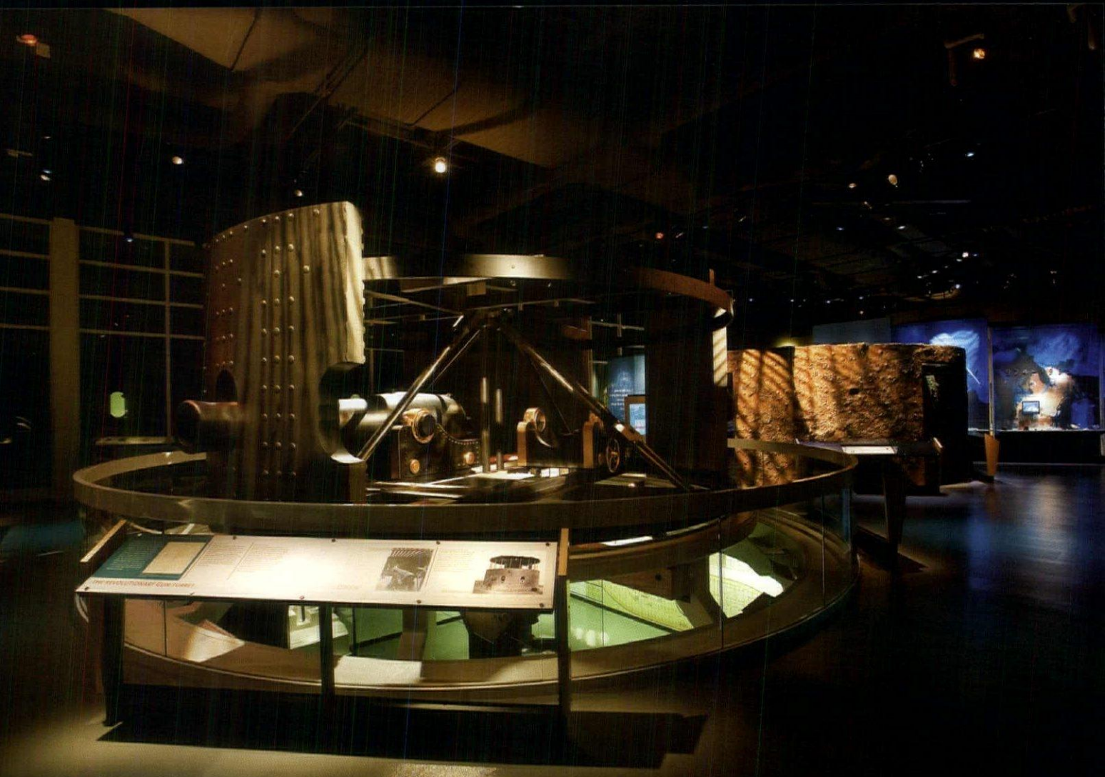
The gallery's dominant leitmotif is the turret, which was 9 feet high, 21.5 feet in diameter and composed of 8 layers of inch-thick iron plating. The rotating turret allowed the ship's cannons to be fired in any direction.
