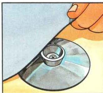
1 Roll membrane over knobbed base plate.
