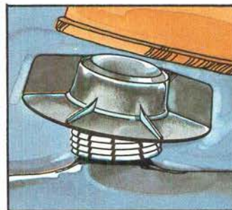
3 Snap and screw on threaded black cap.
