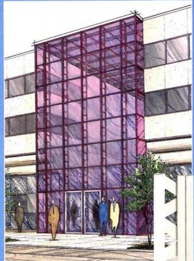
But while the design options offer flexibility, the integrity of the structure remains inflexible. A thermal break, and the flexibility of either 1/4" or 1" glass attest to Trusswall being ready and willing to take on nature's harshest elements.
