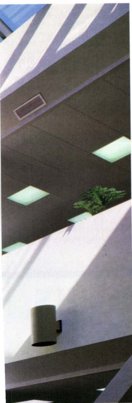
STANDARD GRID with its wide 1\frac{1}{2} " exposed face provides for a ceiling design that is coarse by today's standards. Shown above with standard square-edge lay-in panels.
