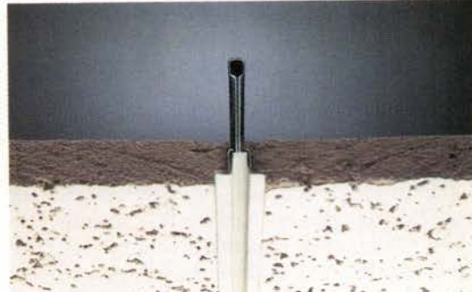
SPECTRA'S narrow \frac{1}{16} " exposed face, cut by a \frac{3}{16} " regress, offers 60% less visible metal at the ceiling plane for a refined look. Shown above with standard square-edge lay-in panels.
