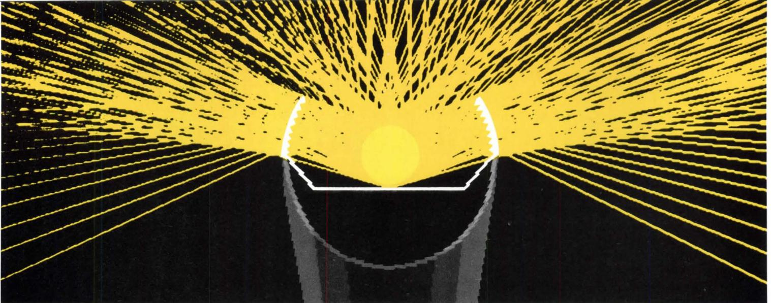
*This six-inch round fixture diffuses light with a proprietary lens system, and the resulting indirect light turns the ceiling into a reflector, creating even light levels and a low glare.*
