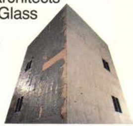
The long-term effects of weather on conventional gypsum sheathing, left; and on Dens-Glass, right.
