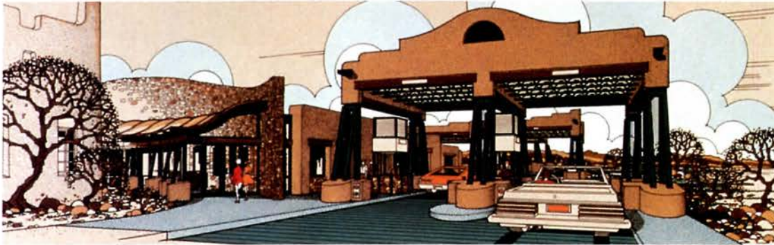
INSPECTION BOOTHS: Copper-roofed canopies incorporate stepped parapets and battered columns of historic structure.
