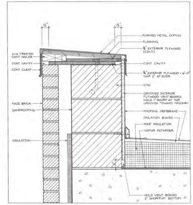
ROOF EDGE VENT DETAIL: Incorporates continuous cavities along front and back.
