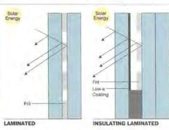
tested on structural glazing. The frit can be translucent or opaque, and the underlying glass clear or tinted, depending on the visual effect and energy control desired. Manufacturers often recommend creating mock-ups, particularly for customized patterns, to test both the visual and sunshading properties of the proposed fritted glazing.
