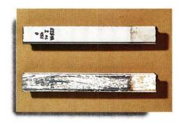
These three year old natural weathering test panels show our high performance finish (top) has far better adhesion and integrity than ordinary conventional paints (bottom).
