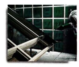
Our trained specialists use spraying techniques that ensure a consistent finish on your products using the most environmentally sound equipment. Minimum film thickness is 3.5 mils. That's thicker than most metal clad products.
