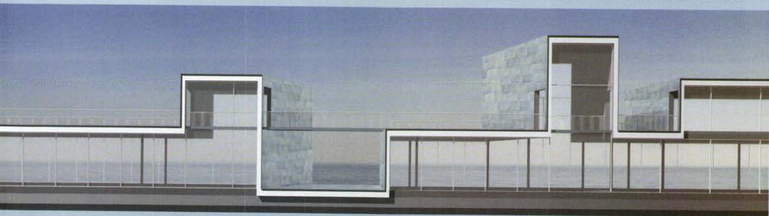
Southeast façade, showing steel cladding on a post-tensioned concrete structure
