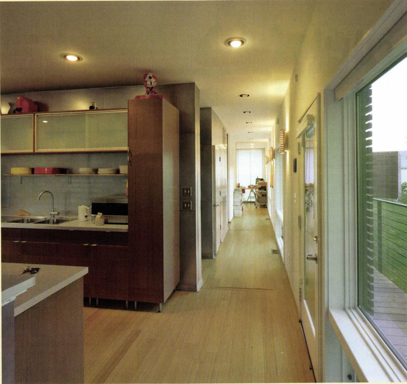
THE MODULES FOR THE KITCHEN (ABOVE) AND FOR THE BATHROOM AND UTILITIES AREA (BELOW) SHARE A WALL FOR EFFICIENT AND ECONOMICAL INSTALLATION OF THE PLUMBING SYSTEM. BOTH SPACES ALSO EMPLOY THE SAME RECYCLED-ALUMINUM WALL COVERING. BAMBOO FLOORING IS USED THROUGHOUT THE HOUSE.
