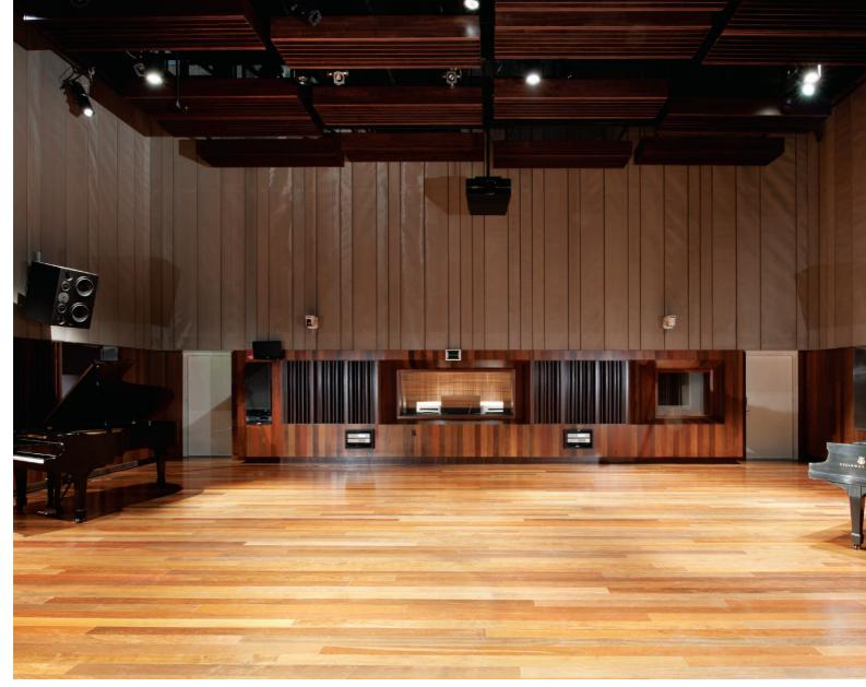
The recording studio-located  $% \left( 1\right) =\left( 1\right) \left( 1\right) \left($ on the south end of the building—is the most acoustically sensitive room in the building. To isolate the room from the rest of the facility, the walls are  $\ensuremath{\mathsf{a}}$ massive 4 feet, 1 inch thick.
