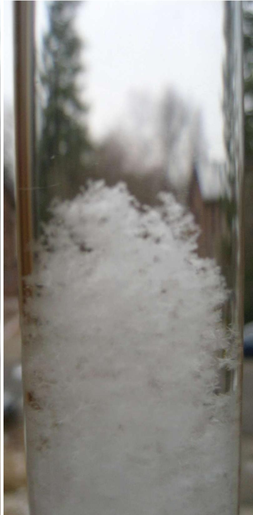
These fluid-filled glass tubes form the basis for Ply Architecture's Stormglass system. The liquid (a formula based on research into the original storm-glass tubes designed in the 18th century) crystallizes in various patterns depending on approaching weather conditions (top).
